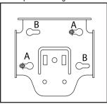
1. With bracket in position in window, mark location where screws should be in either A & A or B & B locations. Screw in fasteners loosely where marked.
