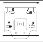
2. Slip the mounting bracket over the two screws and slide the bracket sideways until the screw heads capture the bracket.
