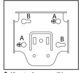
3. After step 2, screws will be seated into small end of slot in bracket. Then tighten these screws completely to secure bracket.
